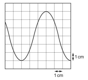
The time-base setting is 0.5 ms cm<sup>-1</sup> and the Y-plate sensitivity is 0.2 mV cm<sup>-1</sup>.
