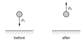
The ball has momentum  $p_1$  downwards just before hitting the ground. After rebounding, the ball leaves the ground with momentum  $p_2$  upwards. The ball is in contact with the ground for 0.020 s. During this time interval, an average resultant force of 25 N acts on the ball.
