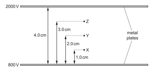
What is the electric field strength, in V m<sup>-1</sup>, at X, Y and Z?
